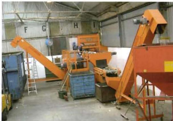
Magnapower Mini MRF Can Sorting Plant which includes: In Feed Hopper, Hand Picking Conveyor, Overband Magnet, Can Flattener, Eddy Current Can Separator, Discharge Conveyors.
